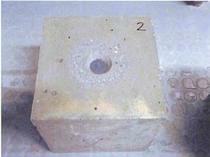
Photo 3: Test object 2 with inserted sealing plug
